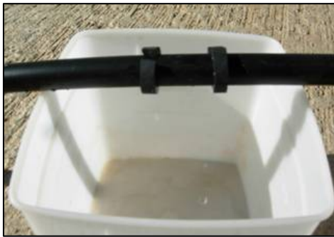
Figure 2. Radiator hose segments placed on tape for flow measurement, one on each side of the emitter. Note the square cornered container that is easy to pour into a graduate cylinder without spilling.
