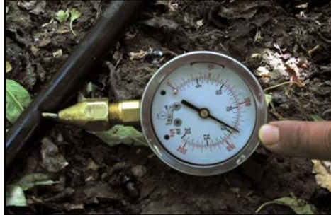
Figure 1. 30 psi oil-filled pressure gauge with pitot tube stuck into tape
