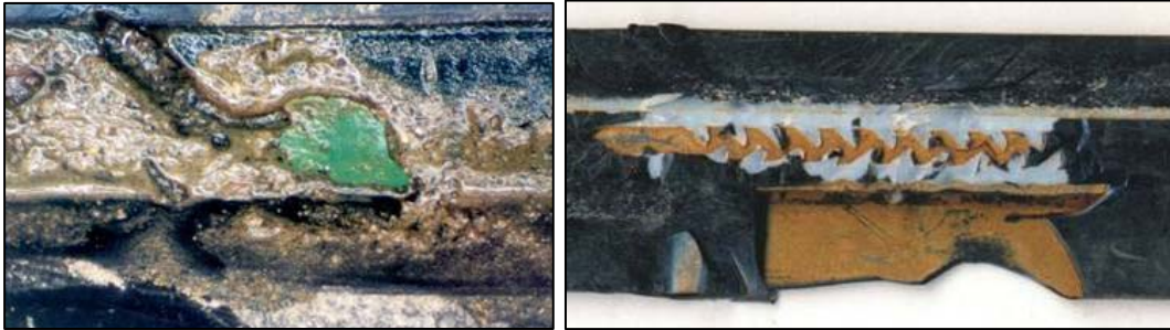
Figure 10. Extreme cases of bacterial slime plus silt and clay (l) and iron deposits (r) plugging an emitter
