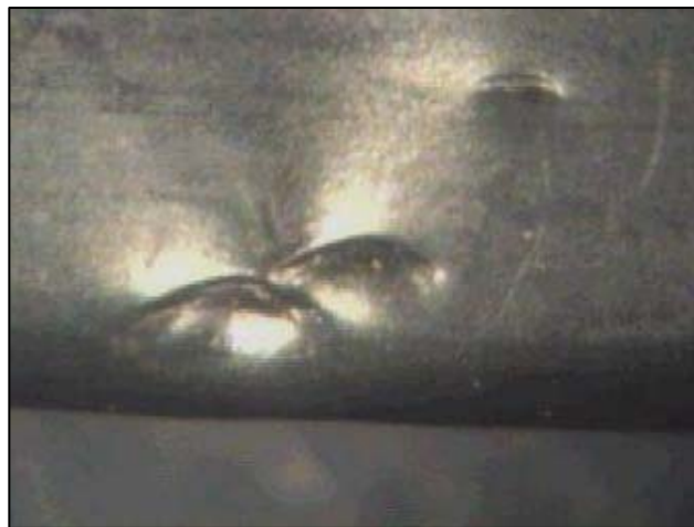
Figure 20. Bird damage on 15 mil tape. The hole is typically somewhat concave inward
