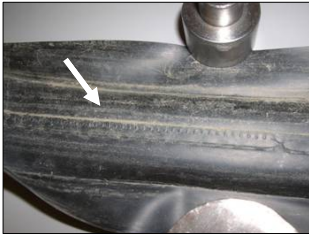
Figure 11. Plugged inlets to the emitter path
